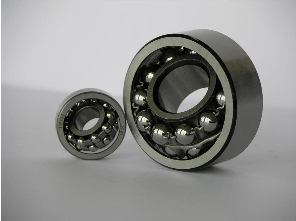
Self-aligning Ball Bearings are designed to contain inner ring and ball assembly in outer ring with a spherical raceway. Due to their special construction, these bearings can tolerate small angular misalignments of shaft up to 2.5 – 3 degrees. These misalignments could either be due to usage, or due to a mounting error.
